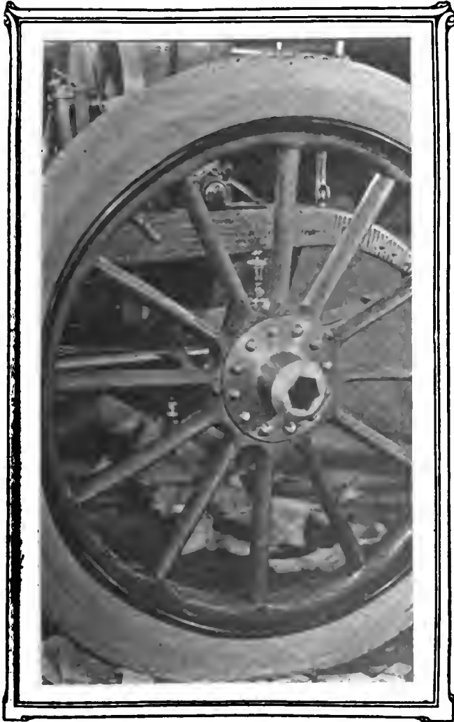
Front wheel of the Oldsmobile, showing hexagon hole in the hub and other nice features in design.
